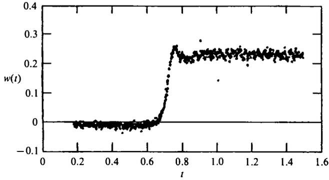
FIGURE 1. Typical raw-data set, showing a discrete time history of the axial-velocity component  $w(t)$ .
