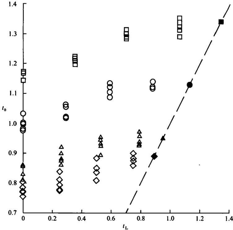
FIGURE 3. Onset times *vs.* laser-delay times for Series II ( $\epsilon = 1.0$ ):  $\square$ ,  $K_I = 0.4$ ;  $\circ$ , 0.6;  $\triangle$ , 0.8;  $\diamond$ , 0.9. Solid symbols indicate average onset times at the limiting condition  $t_L = t_0$ .
