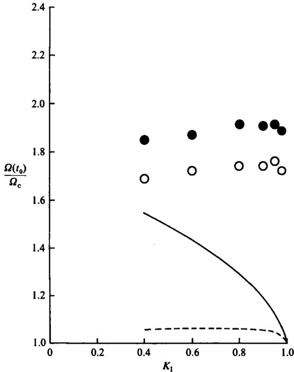
FIGURE 6. Experimental and predicted enhancements for Series III in terms of  $K_I$ :  $\circ$ ,  $\epsilon = 1.6$ ;  $\bullet$ , 3.2. The solid line is the marginal-stability IV prediction for  $\epsilon = 1.6$ ; the dashed line is the absolute-stability IV prediction for  $\epsilon = 1.6$  (Chen *et al.* 1985).
